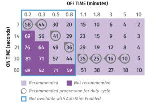
LivaNova recommends that stimulation with Normal Mode ON time > OFF time be avoided. Duty Cycle = (ON Time + 4 seconds) / (ON time + OFF Time), for which ON and OFF Time are measured in seconds.
