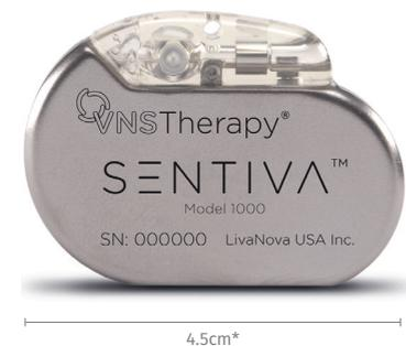
The small **generator** (sometimes called a 'stimulator') is the device that holds the battery and sends signals to the left vagus nerve in the neck through the lead. These signals help to reduce the number and length of seizures.
